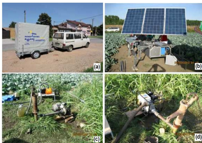
Fig. 21. Disposition of the MSG; (a) in transport, (b) operating position in the cabbage plot, (c) pumping station, (d) pumping unit
