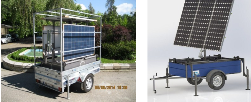
Fig. 14. Dispositions of autonomous mobile solar generator (MSG); close state (left), operating open state (right)
